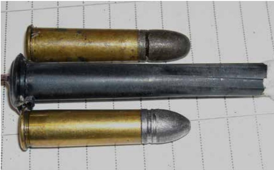
*Top; original factory Cadet round, middle; a chamber cast made of sulphur and graphite powder, bottom; a short case with one of Jeff's cast CBE 325 125 bullets.*
