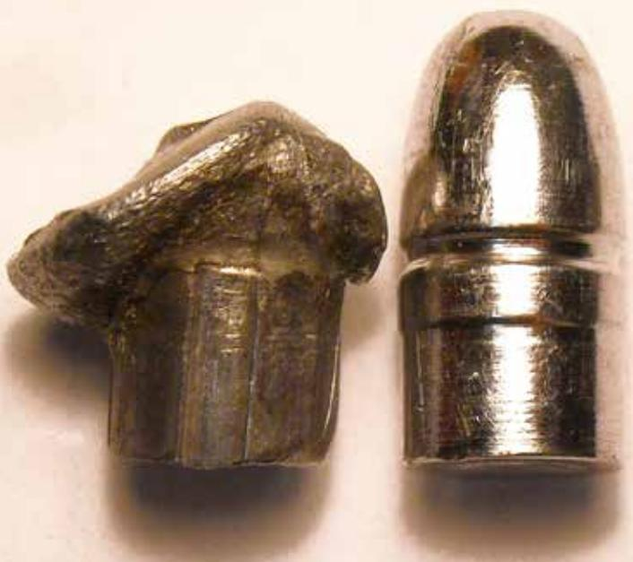
Left; a CBE 320 120 bullet cast in 40-1 alloy recovered from wet phone books at 50 metres. Upon firing the heel has slugged up to groove diameter and there's still some lube left in the groove.
