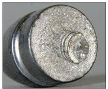
This Linotype alloy bullet was allowed to cool too much and therefore required several blows from the sprue cutting mallet to sever it. Note the small semicircles leading up to the final cut.
