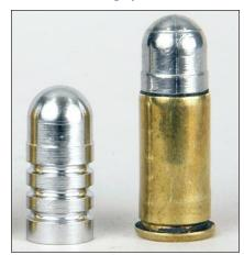
The Lyman 358430 bullet (left) is perfectly formed. The loaded bullet in .38 S&W (right) has some minor wrinkles in its nose that will not be a detriment to accuracy.
