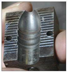
This Minié-ball mould has two problems. The lead speck to the right of the cavity will not allow the mould blocks to close properly. Rust has formed inside the blocks and should be removed with a cotton swab and rust remover.
