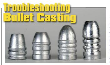
The bullet at far right is simply the result of the mould and/or alloy being too cool. Conversely, the three bullets at left have been poured with a contaminated alloy that does not allow bands and edges to fill out perfectly.
