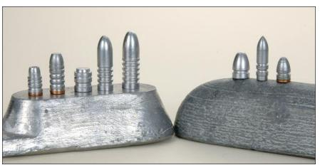
*Mike uses only 1-to-20 (tin-to-lead) foundry alloy for revolver bullets and BPCR bullets (left). For modern rifle bullets and autoloading pistol bullets (right), he uses only Linotype.*
