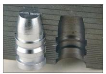
Above, when a mould does not close properly, there will be flashing all around the freshly poured bullet. Below, the mould pin alignment hole on the right can be seen to be slightly peened. That mould is not going to close properly and drop its best bullets until fixed.
