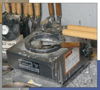
Left, Mike's casting area includes an exhaust fan and a small manicurist's fan (to his left) for cooling sprues. Above, bullet moulds are preheated atop the lead furnace. The same goes for the ladle.
