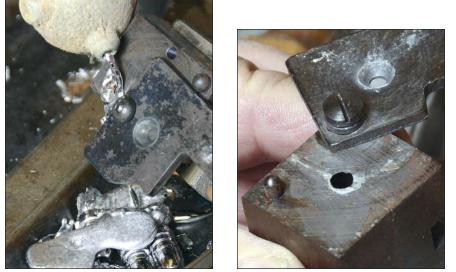
Above, to remove lead smears from atop a set of mould blocks, Mike ladles molten alloy on it until the smear turns shiny. Then it too is molten and can be rubbed off with a piece of cloth. Right, perhaps the most common problem besetting bullet casters is lead smears across the top of moulds. They must be removed for a bullet's base to be perfectly flat.
